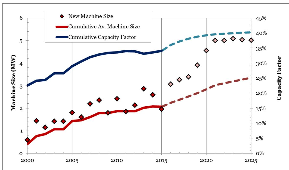
Figure 6 Historical and projected increase in turbine size and average wind farm capacity factor (post losses).
